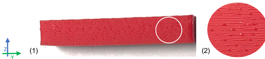
Figure 91 – Scraps on C1 specimens: (1) General and (2) Detailed view.
