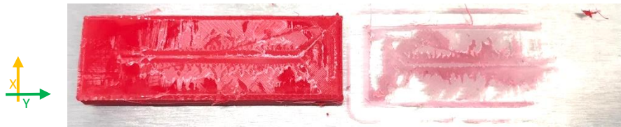
Figure 104 – Bed over-sticking on a H1 specimen.
