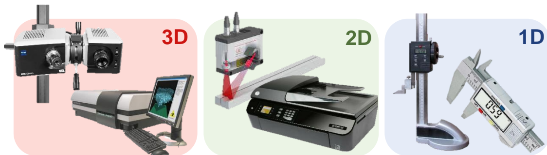
Figure 9 – Warping measuring methods, adapted from [35],[50],[45],[3],[49],[28] accordingly.
