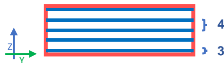
Figure 74 – Illustration (not at scale) of the ironing process with 4 layers in between (C specimens).
