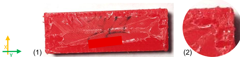
Figure 103 – Bed over-sticking effect on G1 specimens: (1) General and (2) Detailed view.
