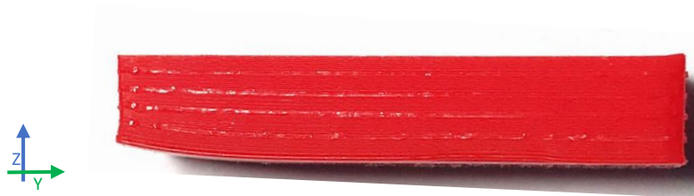
Figure 99 – Ironing traces on E specimens (E1.3).
