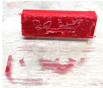
Figure 85 – Specimen with ‘bed over-sticking’.
