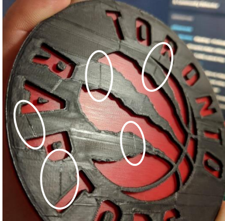
Figure 69 – Undesired ironing lines on a FFF print [78].
