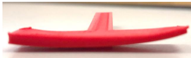
Figure 65 – Warped specimen with h=0.1\text{mm} .
