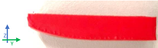
Figure 71 - Results for tests with ironing and h=0.1\text{ mm} .
