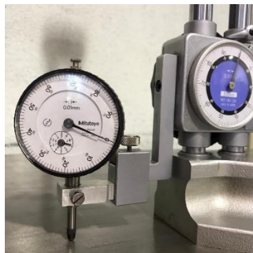
Figure 42 – Comparator's reset to the precision table.
