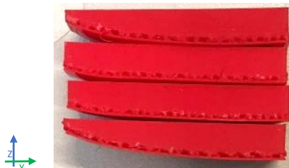
Figure 101 – Melted layers on F1 specimens.
