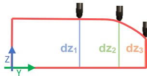
Figure 38 – Illustration of the comparator's measurement on a warped specimen.
