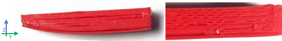
Figure 96 – Stratified warping on D specimens.
